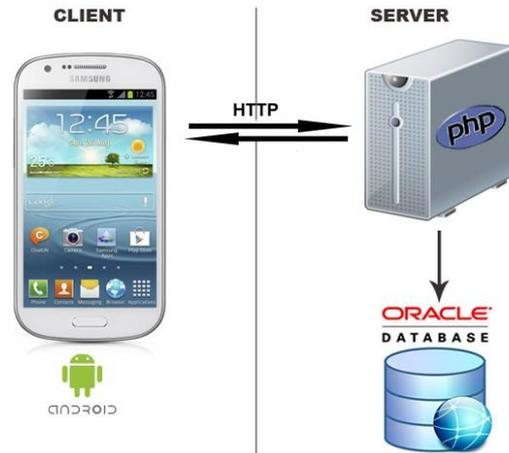
Figure 2. Architecture of the mobile application
