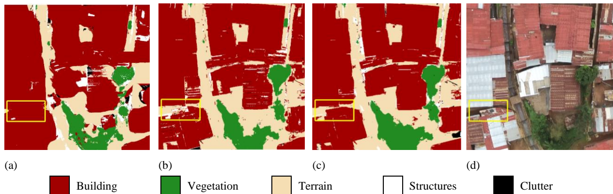
Figure 1. Sample classification results of the RD (a), R2ST (b) and R2ST_all (c) feature sets for the 5-class problem, with the RGB reference image (d). The yellow boxes indicate footpaths that are misclassified as buildings in RD due to DSM errors.
