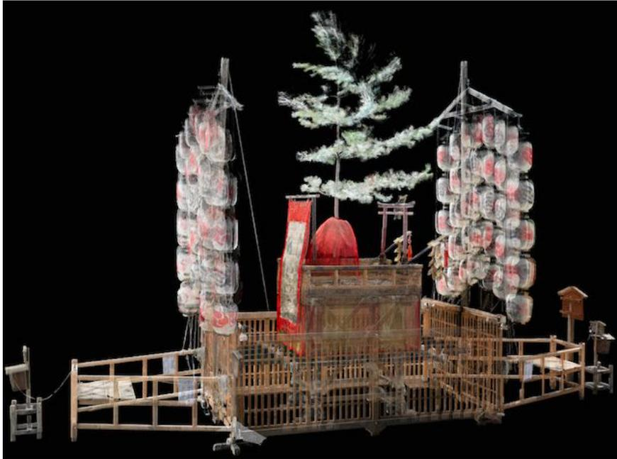
Figure 1. See-through imaging of a laser-scanned point cloud of the Hachiman-Yama float used in the Gion Festival
