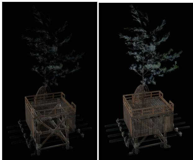
Figure 7. Assignment of different opacities to constituent point clouds in the transparent fused visualization. For the outer box-shaped portion,  $\alpha$  is 0.05 (small) in the left image, and  $\alpha$  is 0.2 (larger) in the right image. For the inner portion,  $\alpha$  is 0.8 in both images. The left image is suitable for observing the inner structure, whereas the right image is suitable for visualizing the outer shape.
