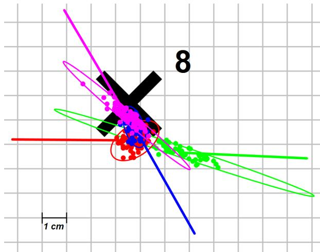
Figure 6: Deviation of calculated positions based on different scans. Different colors show different scanner orientations (black cross: reference position).
