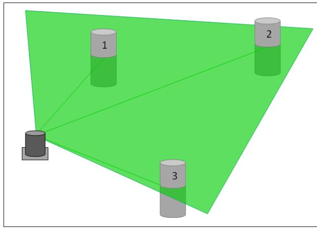
Figure 1: Laser scanner scanning in one horizontal plane.
