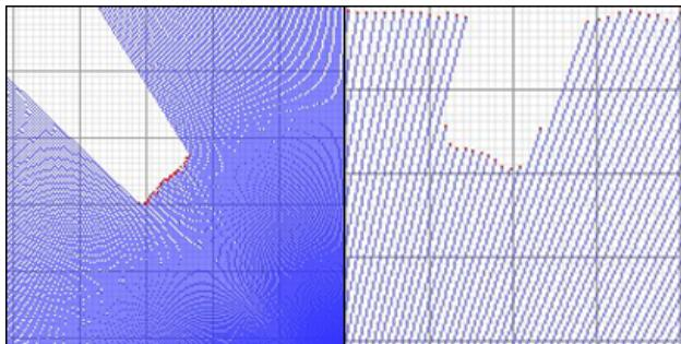
Figure 3: Scan lines plotted for a pole with 110 mm diameter at different distances to sensor (left: approx. 500mm, right: approx. 1500 mm).
