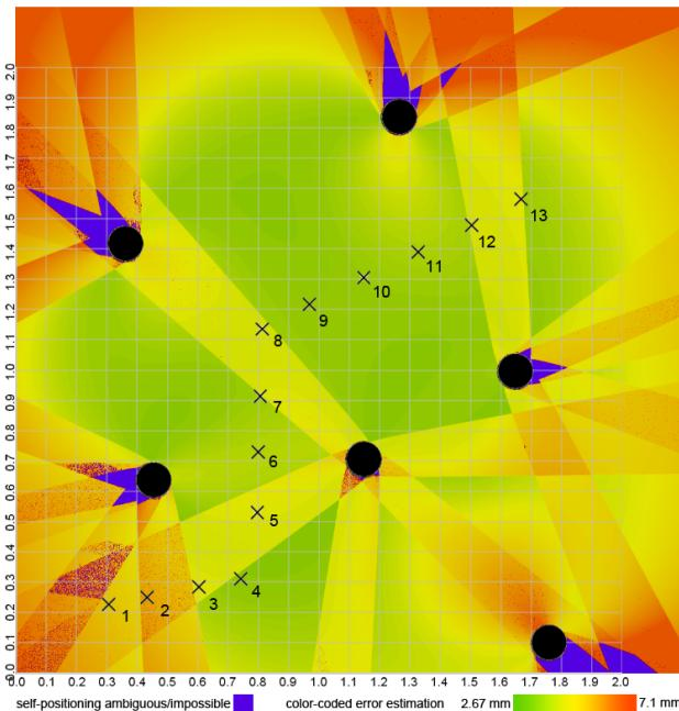
Figure 4: Accuracy color map for one landmark constellation (gray circles) and example trajectory.
