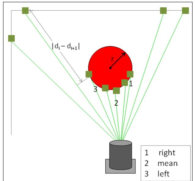
Figure 2: Diagram of depth-jumps at a single pole object.
