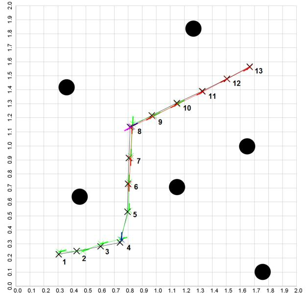
Figure 5: Example trajectory with landmarks. Reference positions are marked as black cross, starting at position 1, green marks forward positions and red backwards positions. Blue and magenta indicate additional directions at turning points.
