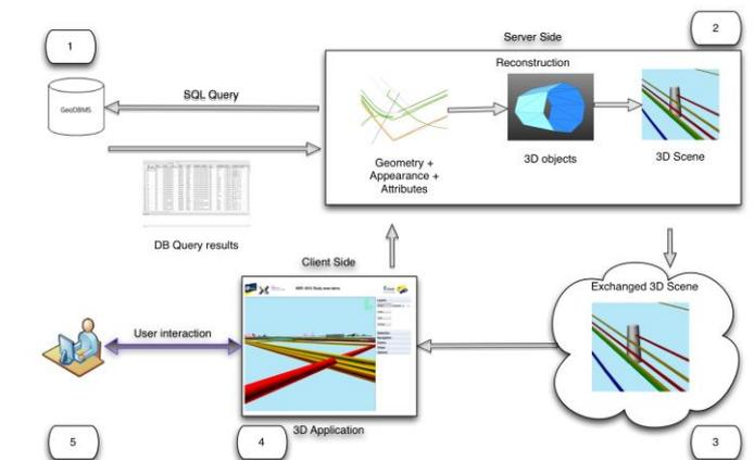
Figure 1: 3D reconstruction flow for pipe lines and cables
