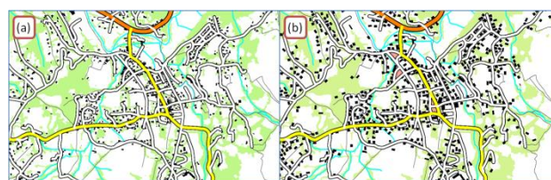
Figure 13. A small town at 1:50k before and after generalization, reducing blank space in the map
