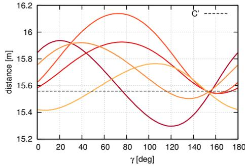
Figure 6:  $d(\tilde{C}', \gamma, Q'_o)$  as a function of  $\gamma$  for five random points  $\tilde{C}'$  in the neighborhood of  $C'$ . The ellipse  $Q'_o$  is the outer circle projection of a target placed a true distance of 15.56 m.
