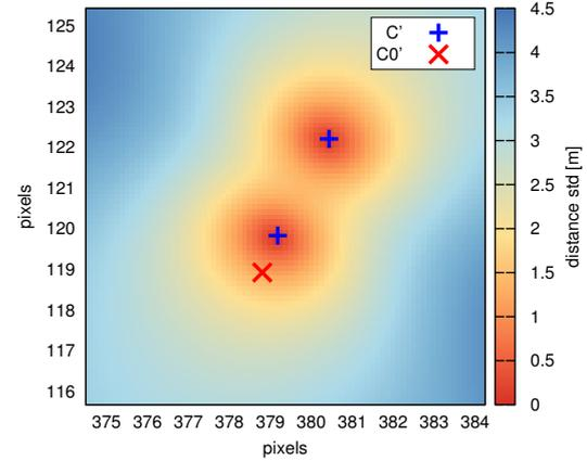
Figure 7: Landscape of  $D(\tilde{C}')$  for an ellipse with major and minor axis 91.02 and 76.46 px, angle  $-113.81^\circ$  and center (379.43, 120.55). Marked points are the two candidates for the projected circle center  $C'$  and the solution obtained employing the method in (Kim et al., 2005).
