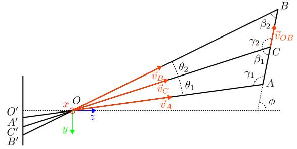
Figure 5: Target pose determination problem, projection on the  $yz$  plane of the camera frame.  $O$  is the camera optical center,  $C$  is the target center and the segment  $\overline{AB}$  is the target diameter which is coplanar to the  $y$  axis. Clearly  $\overline{AC} = \overline{BC} = r$ .
