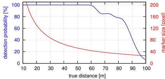
Figure 8: Estimate of the detection probability as a function of the true distance from the camera.
