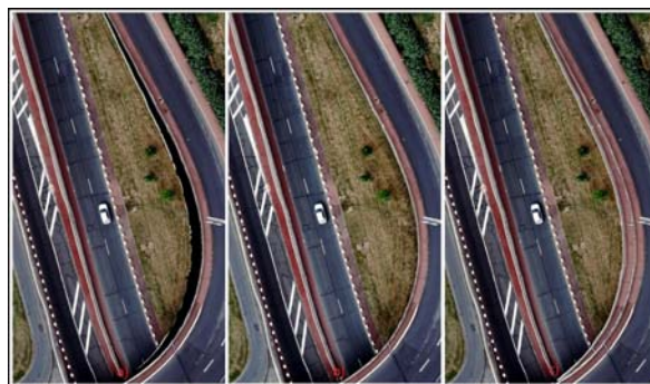
Figure 7. a) Occlusion detection, b) true ortho (with DSM) and c) traditional ortho (with DSM) images (Paris)
