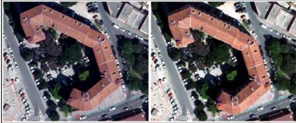
Figure 8. a) True ortho (with DSM) and b) traditional ortho images (with DTM) overlaid with roof models (Toulon)
