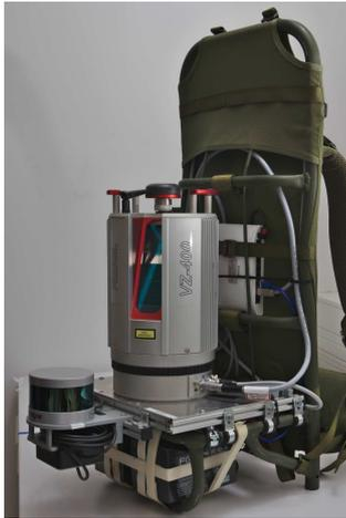
Figure 2. The backpack with Riegl VZ-400 and Velodyne VLP16 Lite laser scanners
