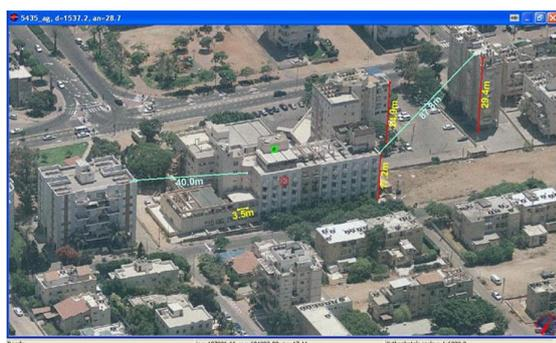
Figure 5. Height and distance measurements (Aeromap, 2006)
