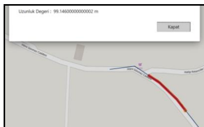
Figure 12. Approximate measurement of road disturbance record by measurement tool
