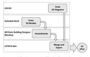
Figure 7. defined steps and utilised software for creating a 3D ePlan
