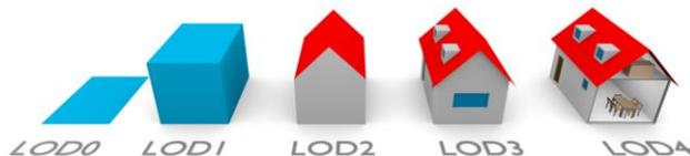
Figure 1. The levels of detail for buildings in CityGML (Biljecki et al., 2016)
