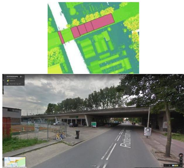
Figure 5. Buildings under bridges have no corresponding heights in AHN. Picture from © Google
