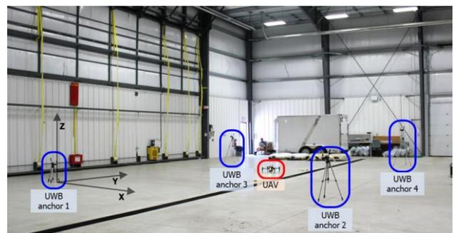
Figure 6. Experimental setup, showing the configuration of UWB anchors
