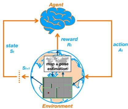
Figure 1. Proposed framework combining reinforcement learning and SLAM where the reconstructed 2D map and the pose estimation of the SLAM algorithm contributes to both state estimation and reward shaping process. As a result, the agent can choose the best action to steer the robot and to support the continuation of the active SLAM algorithm.
