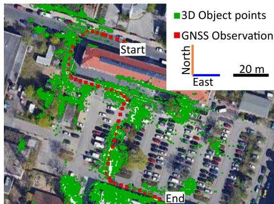
Figure 3. The trajectory driven by the two vehicles, represented by the GNSS observations and the 3D tie points. A satellite image of the area is used as background.
