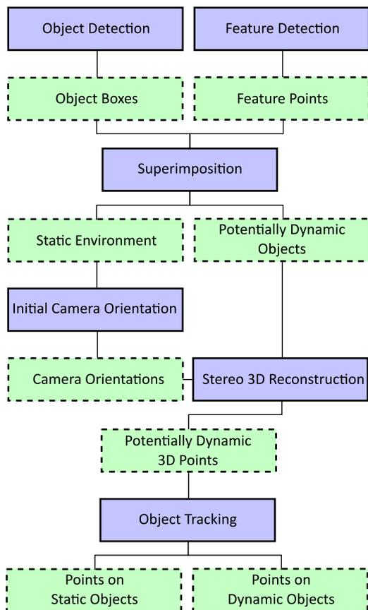
Figure 1. This flowchart shows the procedure used in this paper to identify points on dynamic objects. Blue solid boxes refer to processing steps and green dashed boxes to data.
