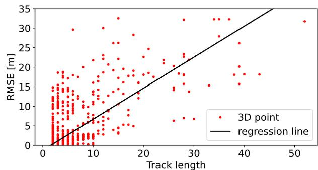
Figure 6. Relation between the track length given by the number of observations of a 3D point, and the RMSE of the position of potentially dynamic 3D points.
