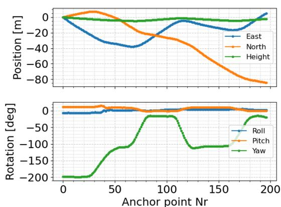
(a) Exterior orientation of the vehicle as a function of time. Top: Position (East, North and Height). Bottom: Rotation angles (roll, pitch, yaw).
