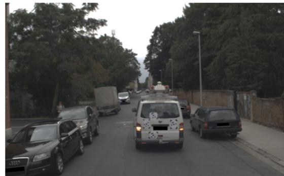
Figure 4. Image taken by one of the cameras of the *vehicle* at the beginning of the trajectory; the vehicle corresponding to the *dynamic GCP* can be seen in the centre of the image.
