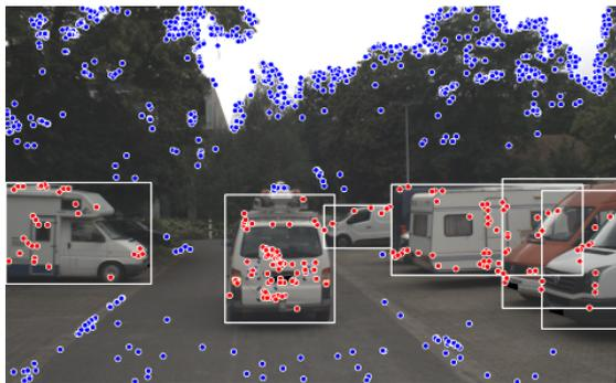
Figure 5. Result of the extracted potentially dynamic objects superimposed with the detected feature points. *Blue*: Feature points in the static environment. *Red*: Feature points situated on potentially dynamic objects.
