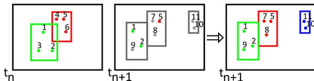
Figure 2. Propagation of object IDs from one frame to the next. Point IDs are shown by a number and object IDs by colour, *grey* indicates that no object ID is assigned.
