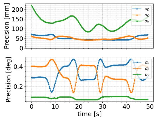
(b) Precision of the exterior orientation parameters resulting from Scenario 1. Top: Position (driving  $\sigma_D$ , orthogonal  $\sigma_O$  and vertical  $\sigma_V$ ). Bottom: Rotation angles (roll  $\sigma_R$ , pitch  $\sigma_P$  and yaw  $\sigma_Y$ ) angle.
