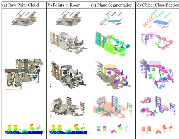
Figure 5. Qualitative results of indoor object classification. (a) Original data (certain datasets have the ceilings removed for clarity). (b) Side view of data in one room. (c) The patch segmentation result of one room. (d) The classification results in one room (One colour represents one type of objects).
