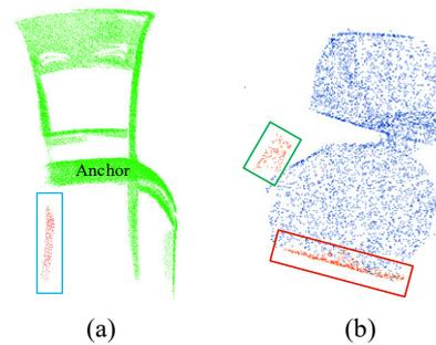
Figure 4. The unclassified cases: (a) missing parts in the chair leg (blue box), (b) the anchor over-segmentation (red box) and chair's tiny parts (green box).
