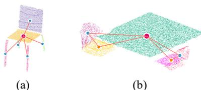
Figure 1. The anchor-based graphs: (a) the graph of one chair, where red node represents the anchor  $v^A$  and yellow line between red node and blue node represents edge; (b) the graph of a sub-scene with one table and two chairs, where yellow node represents the sub-anchor  $v^{SA}$ .
