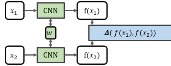
Figure 2. Siamese architecture. Two images are propagated through the same CNN architecture. Both CNNs share their weights  $w$ . The L2 distance  $\Delta$  of the resulting feature vectors  $f(x_1), f(x_2)$  is used to calculate the training loss.
