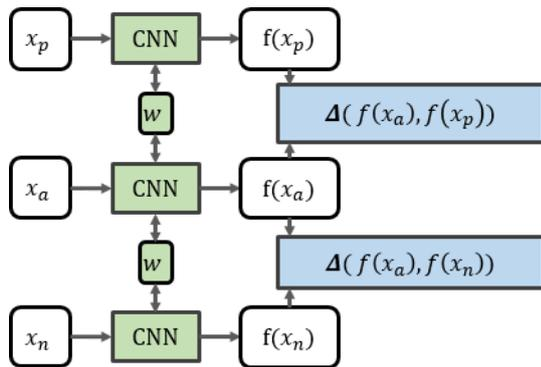
Figure 3. Triplet architecture. Three input images are propagated through the same CNN architecture. The CNN branches share their weights  $w$ . The L2 distances  $\Delta(f(x_a), f(x_p))$  and  $\Delta(f(x_a), f(x_n))$  of the resulting feature vectors are the basis for calculating the loss to be minimized in training.
