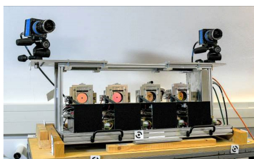
Figure 8. High-speed cameras mounted on fan-shaped distance meter system
