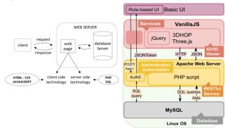
**Figure 2.** System architecture of METEORA platform. Left: Client-side to server-side communication. Right: Technological tools and interactions of the 3-Tier Architecture model.
