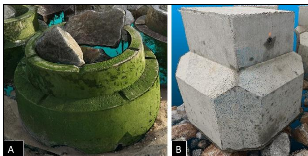
Figure 1. A: Accroberm™ II (2.24 m diameter); B: 'double cube' unit (1.3 m nominal diameter)
