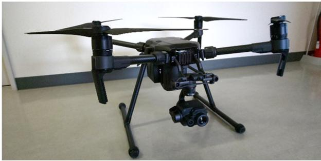
Figure 2. UAS utilized in this work (Matrice 210 and Zenmuse-XT2).
