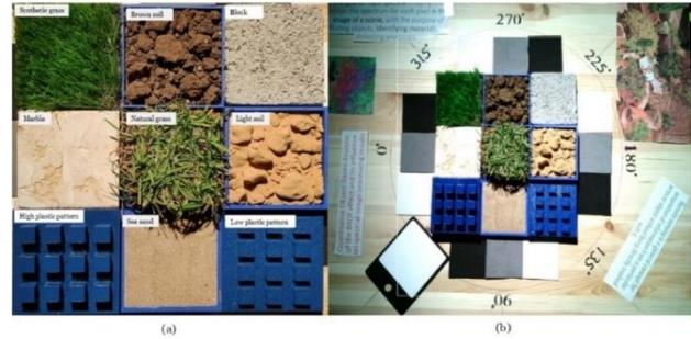
**Figure 2.** The nine different materials used in experiment (a) were placed on top of a wooden plate marked with a circle of azimuths (b).
