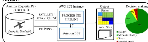
**Figure 2.** Top-level architecture of ADDPro pipeline
