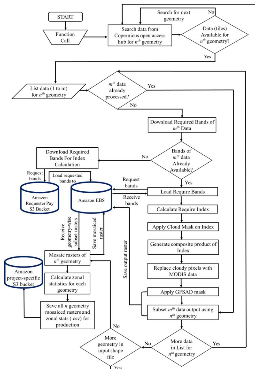
Figure 3. Detailed process flow diagram of ADDPro pipeline
