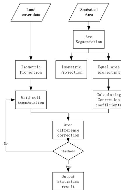
**Figure 7.** Flowchart of the developed strategy to correct the area distortion
