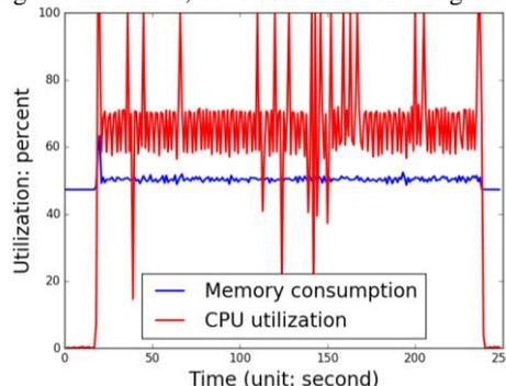
Figure 12 Result of robustness experiment. The x-axis is the elapsed time and y-axis is the percentage of usage of computer memory and CPU. The red line denotes the consumption of the
