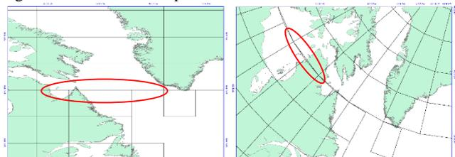
**Figure 1** Demonstration of errors from projection schemes. (a) Geographic coordinate system; (b) UTM projection (a type of isometric projection). The red line circles the identical region in both geographic coordinate system and after UTM projection, to show errors in area-size after isometric projection.
