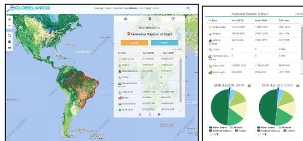
**Figure 8** Demonstration of the user requests in GlobeLand30 GSA. (a) The user request and corresponding the land cover analysis result; (b) the analysis result of the land cover change between 2000 and 2010.
