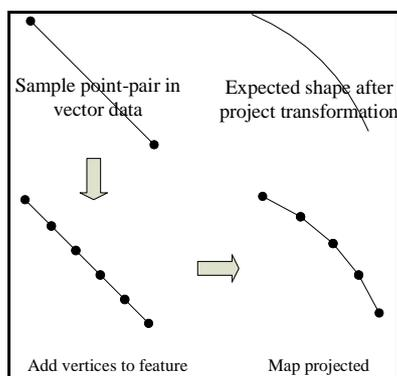
**Figure 6.** Demonstration of projective deformation errors and the correction algorithm with differential geometry theory.
