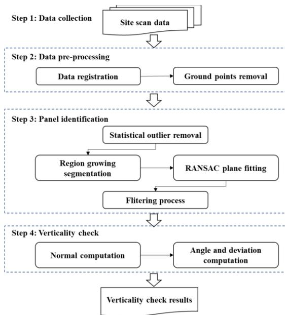
**Figure 1.** Framework of verticality check approach.
